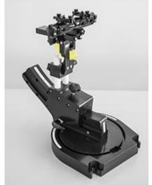
which the devices must be measured are defined by the standards. The DASY device holder is designed to cope with the different positions given in the standard. It has two scales for device rotation (with respect to the body axis)
