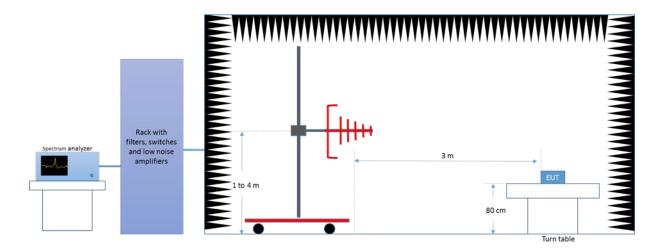
Radiated Setup 1 GHz - 6.4 GHz
