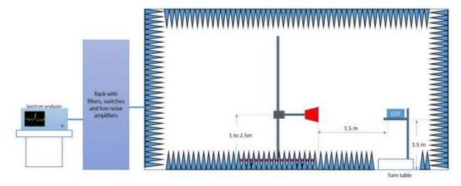
Radiated Setup 6.4GHz - 18 GHz
