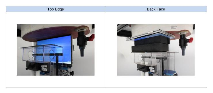
F.3 Antenna host platform location and adjacent edge positions relative to the body
