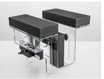
A simple but effective and easy-to-use extension for the Mounting Device; facilitates testing of larger devices according to IEC 62209-2 (e.g., laptops, cameras, etc.); lightweight and fits easily on the upper part of the Mounting Device in place of the phone positioner. The extension is fully compatible with the Twin SAM, ELI and other Flat Phantoms.
