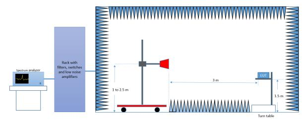
Radiated Setup 18 GHz – 40 GHz
