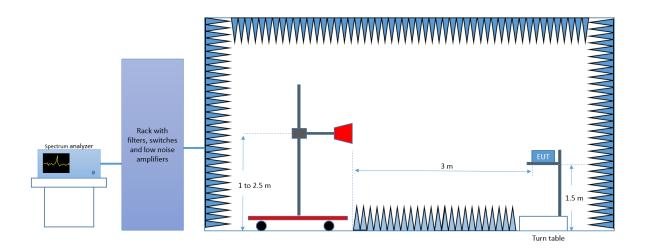
Radiated Setup 18 GHz - 40 GHz
