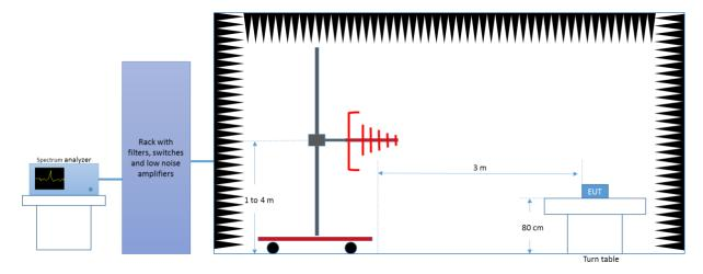
Radiated Setup 1 GHz - 18 GHz
