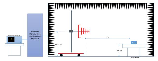
Radiated Setup 1 GHz - 18 GHz
