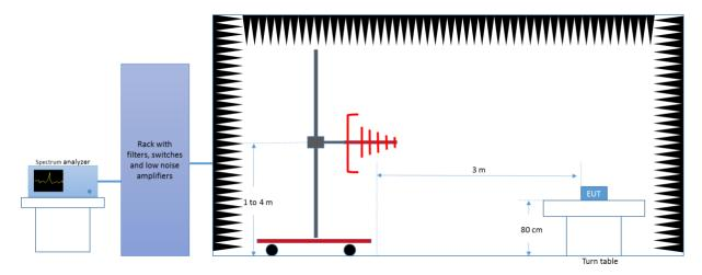
Radiated Setup 1 GHz - 18 GHz
