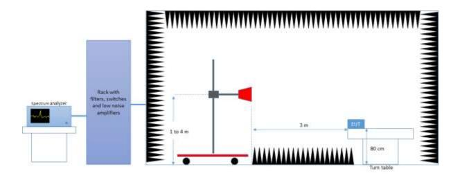
Radiated Setup 18 GHz - 40 GHz
