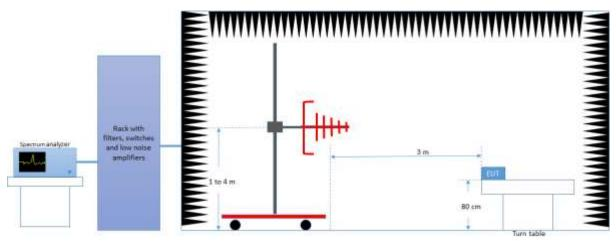
Radiated Setup 1 GHz - 18 GHz
