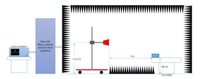
Radiated Setup 18 GHz - 40 GHz
