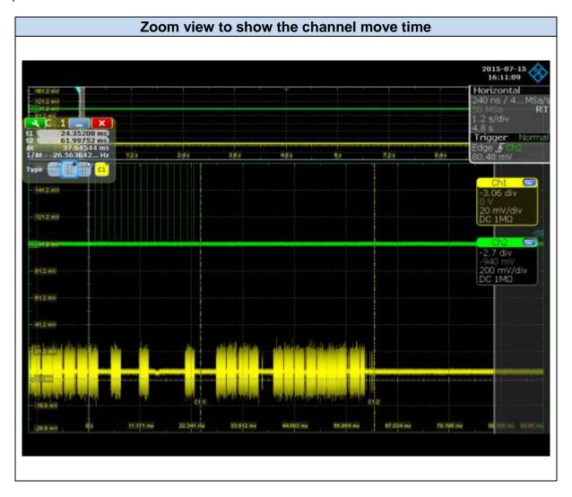
On the screenshot above, the cursors are placed between the latest radar signal and the latest data packet transmitted by the EUT to the master device. The time delta value show the channel move time, here the value is 37.65 ms.
