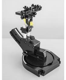
The DASY devices must be measured are defined by the standards. The DASY device holder is designed to cope with the different positions given in the standard. It has two scales for device rotation (with respect to the body axis) and device inclination (with respect to the line between the ear reference points). The rotation center for both scales is the ear reference point (ERP). Thus the
