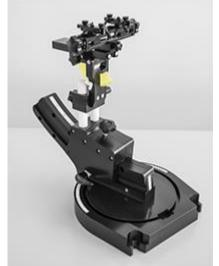
which the devices must be measured are defined by the standards. The DASY device holder is designed to cope with the different positions given in the standard. It has two scales for device rotation (with respect to the body axis) and device inclination (with respect to the line between the ear reference points).
