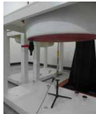
Photo of the dipole Antenna
