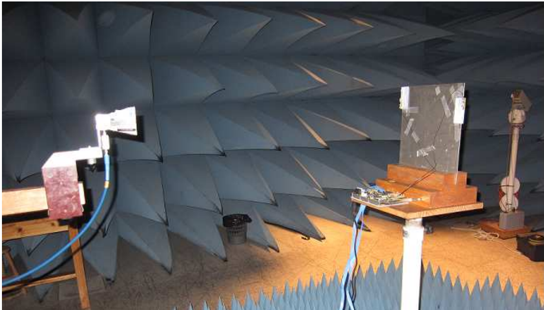
Fig. 4. Test set-up for radiated measurements above 30MHz to 18GHz
