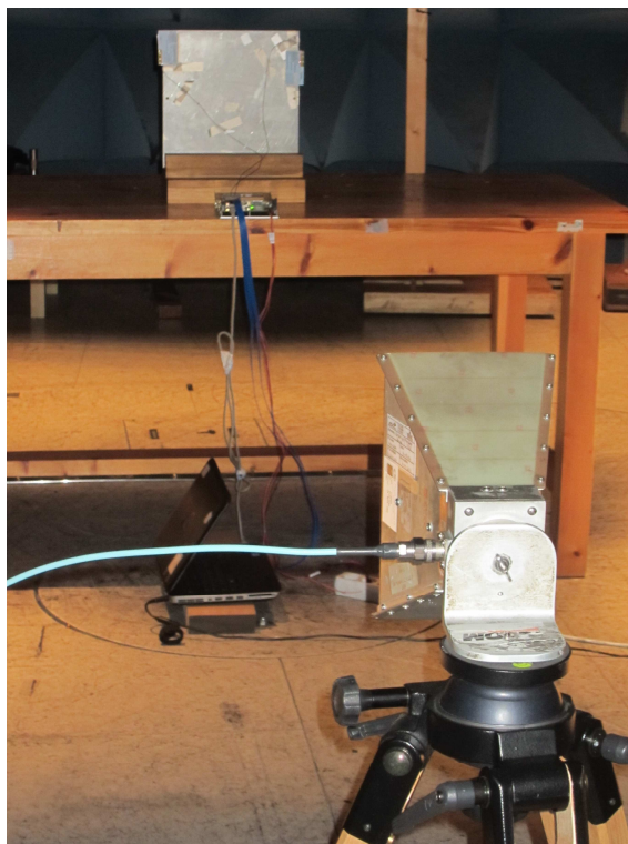
Fig. 4. Test set-up for radiated measurements above 30MHz to 1GHz
