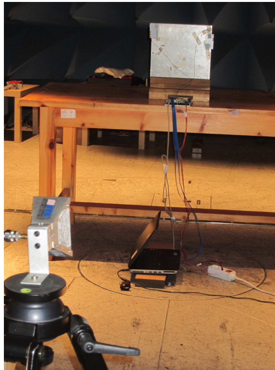
Fig. 6. Test set-up for radiated measurements above 18GHz to 26GHz
