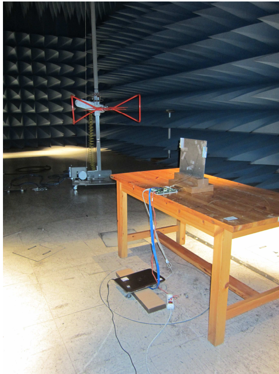
Fig. 4. Test set-up for radiated measurements above 30MHz to 1GHz
