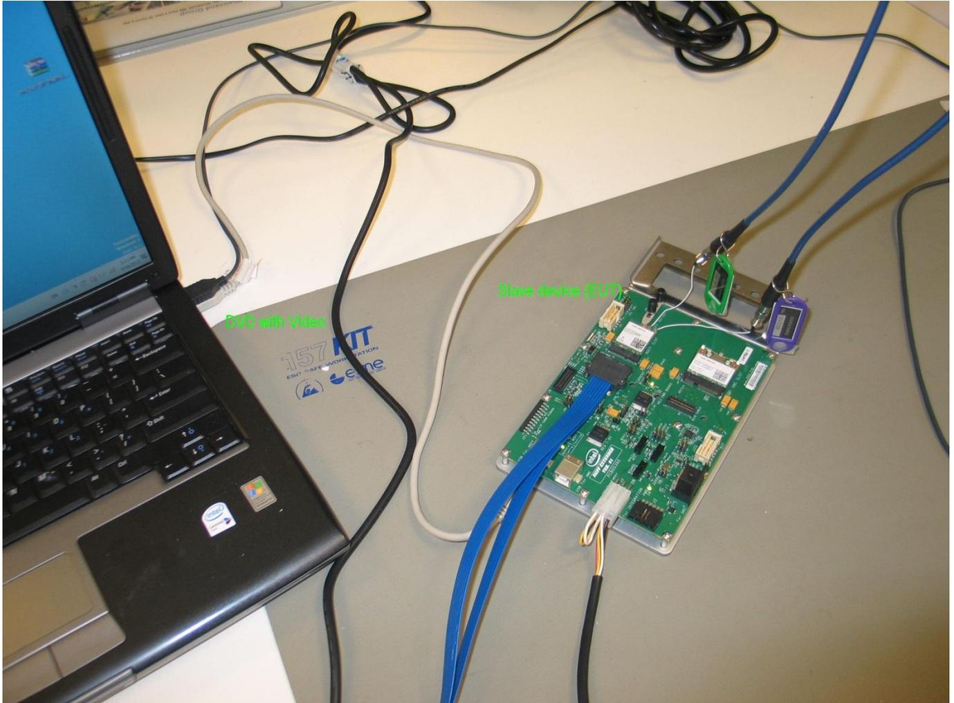
*EUT setup with laptop and DVD with Video. The video is displayed via the RF connection to the Access Point on a second laptop*
