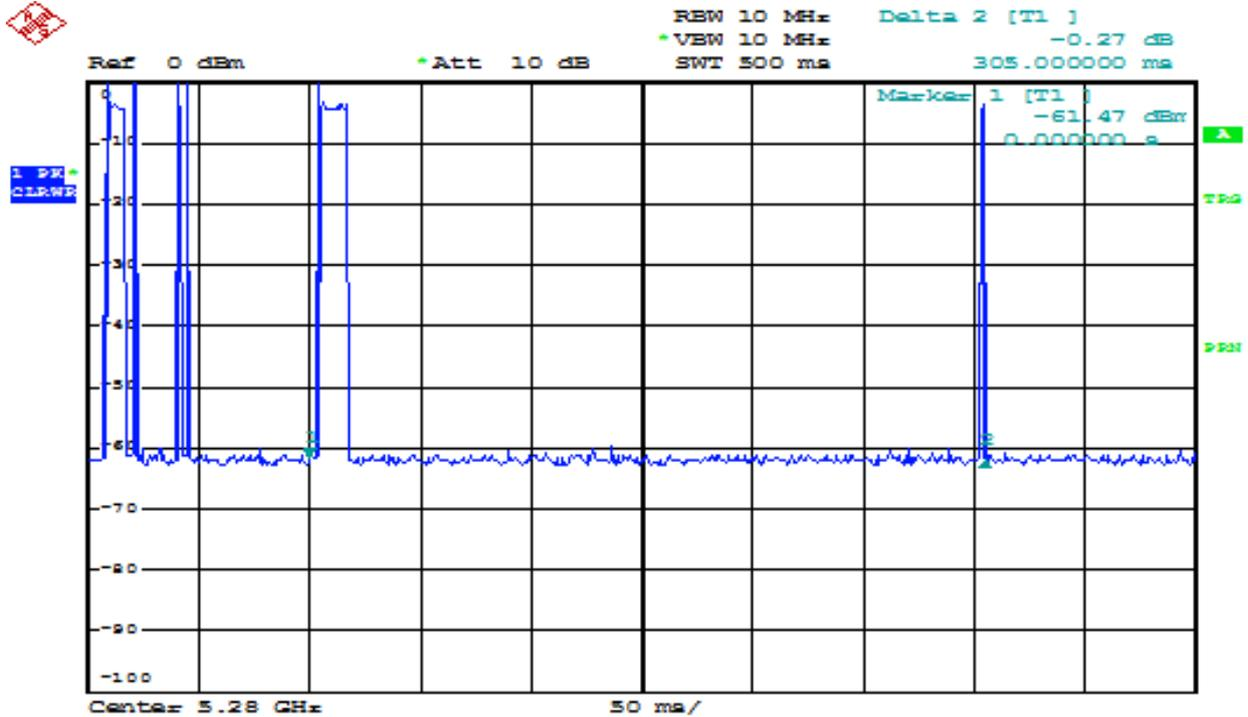
Channel move time (Marker 1 represents end of the radar pulse)
