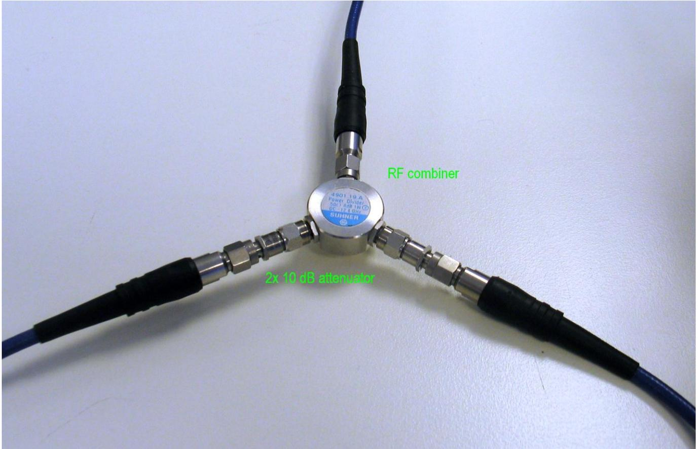
*Combiner and 2x 10 dB attenuator to combine the two antenna ports of the EUT. The output of the combiner is connected to the spectrum analyzer. The If output of the spectrum analyzer is connected to the DFS testtool.*
