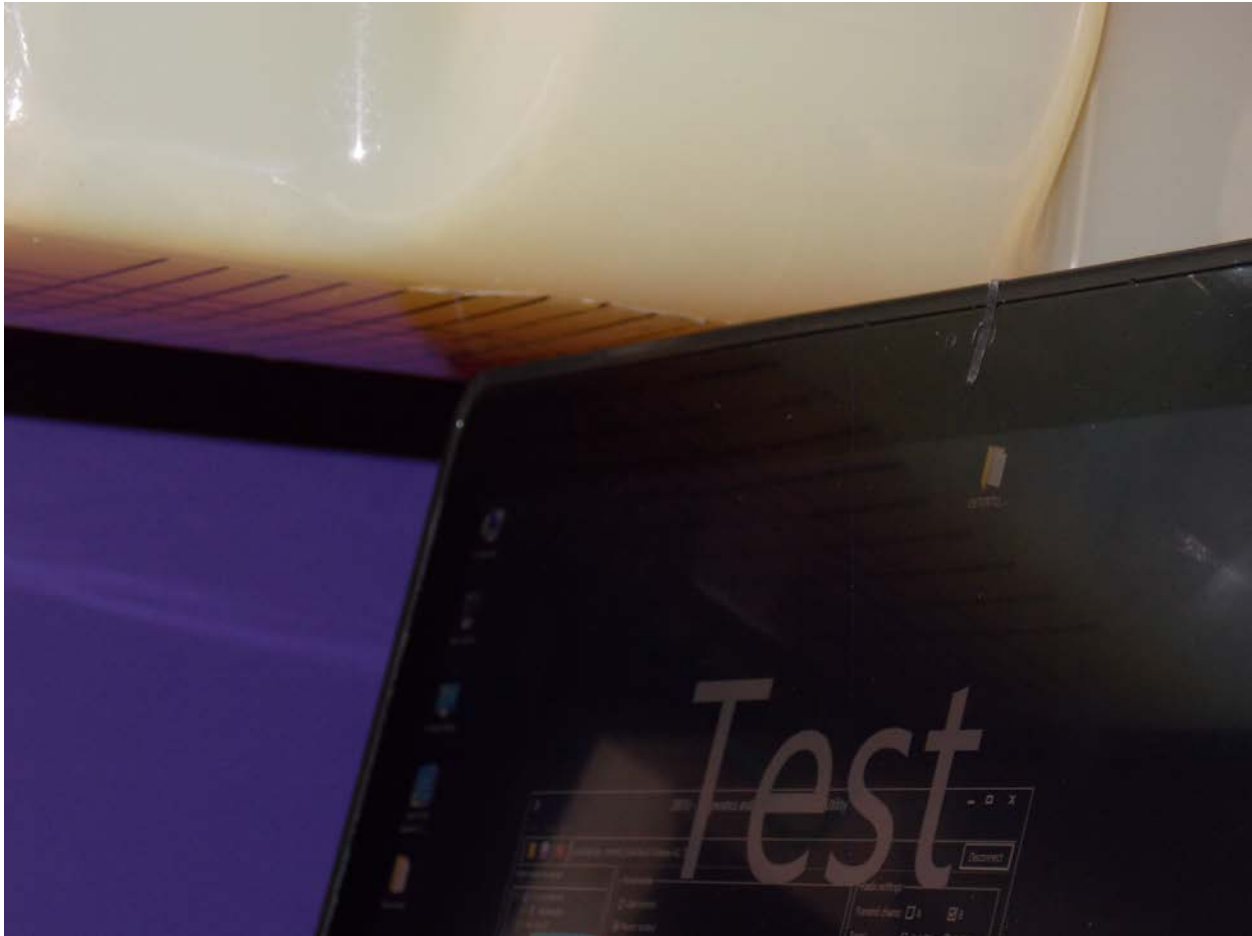
Test Position Secondary Landscape Main Antenna 0 mm Gap
