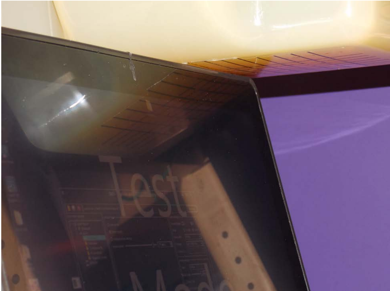
Test Position Secondary Landscape Aux Antenna 0 mm Gap
