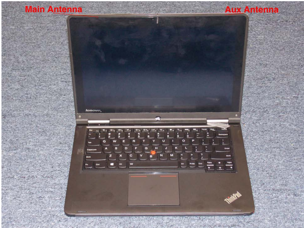
Laptop Mode and Antenna Location
