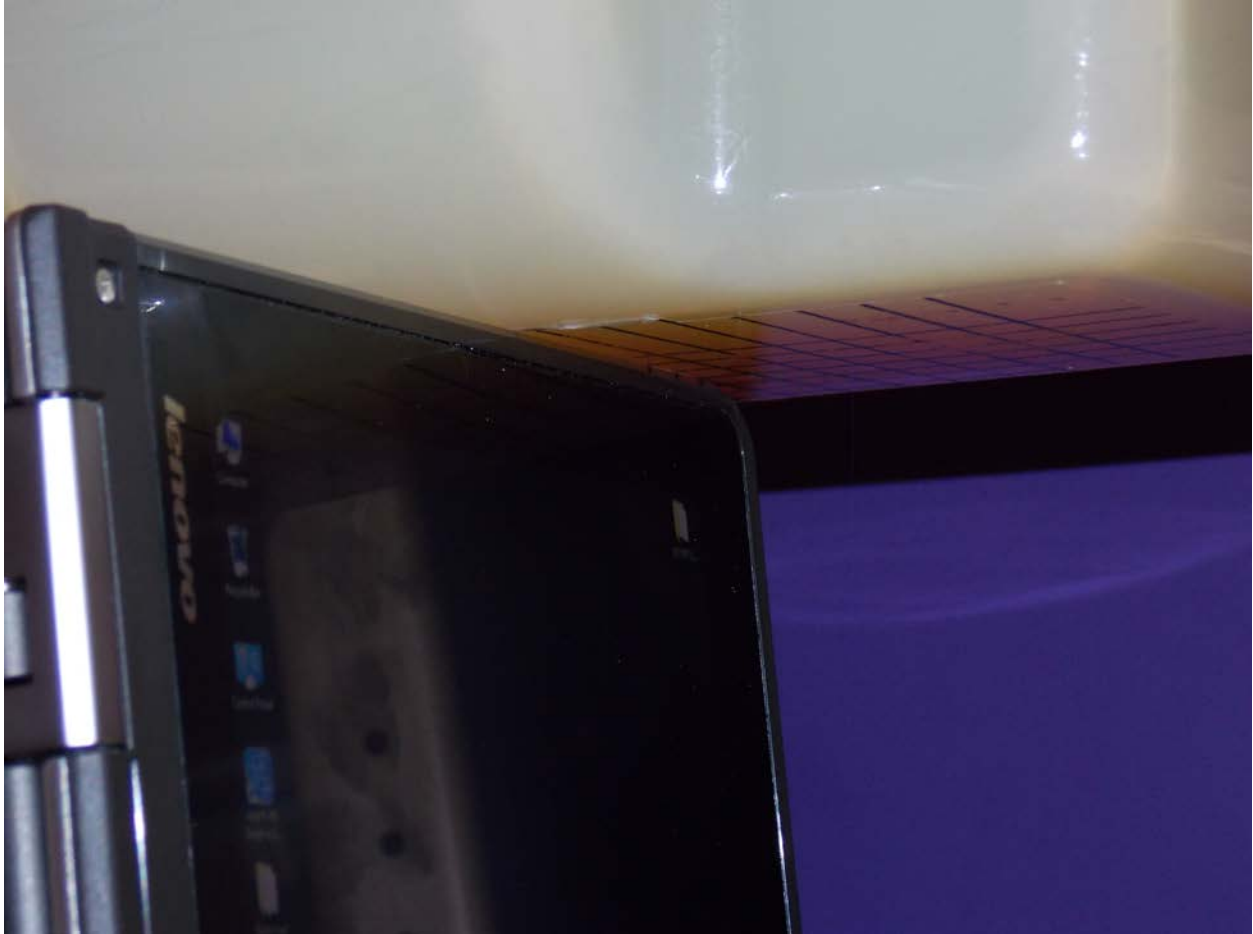
Test Position Primary Portrait Main Antenna 0 mm Gap
