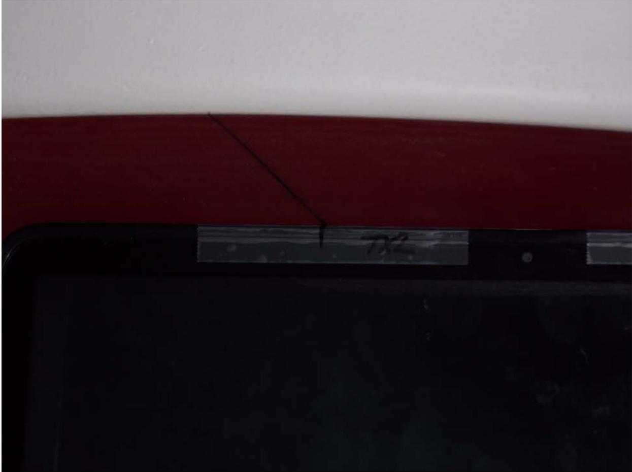
**Test Position Tablet Mode Top Side 0 mm Gap**
