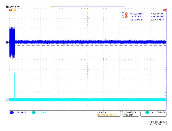
The upper trace in the above plot has 10 seconds of EUT final transmission data and the lower trace shows the simulated radar signal.
