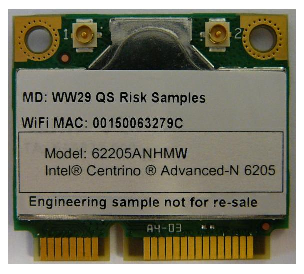
Photo showing label placement on half-mini card.
