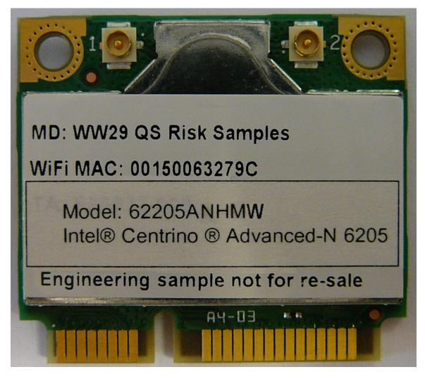
Photo showing label placement on half-mini card.
