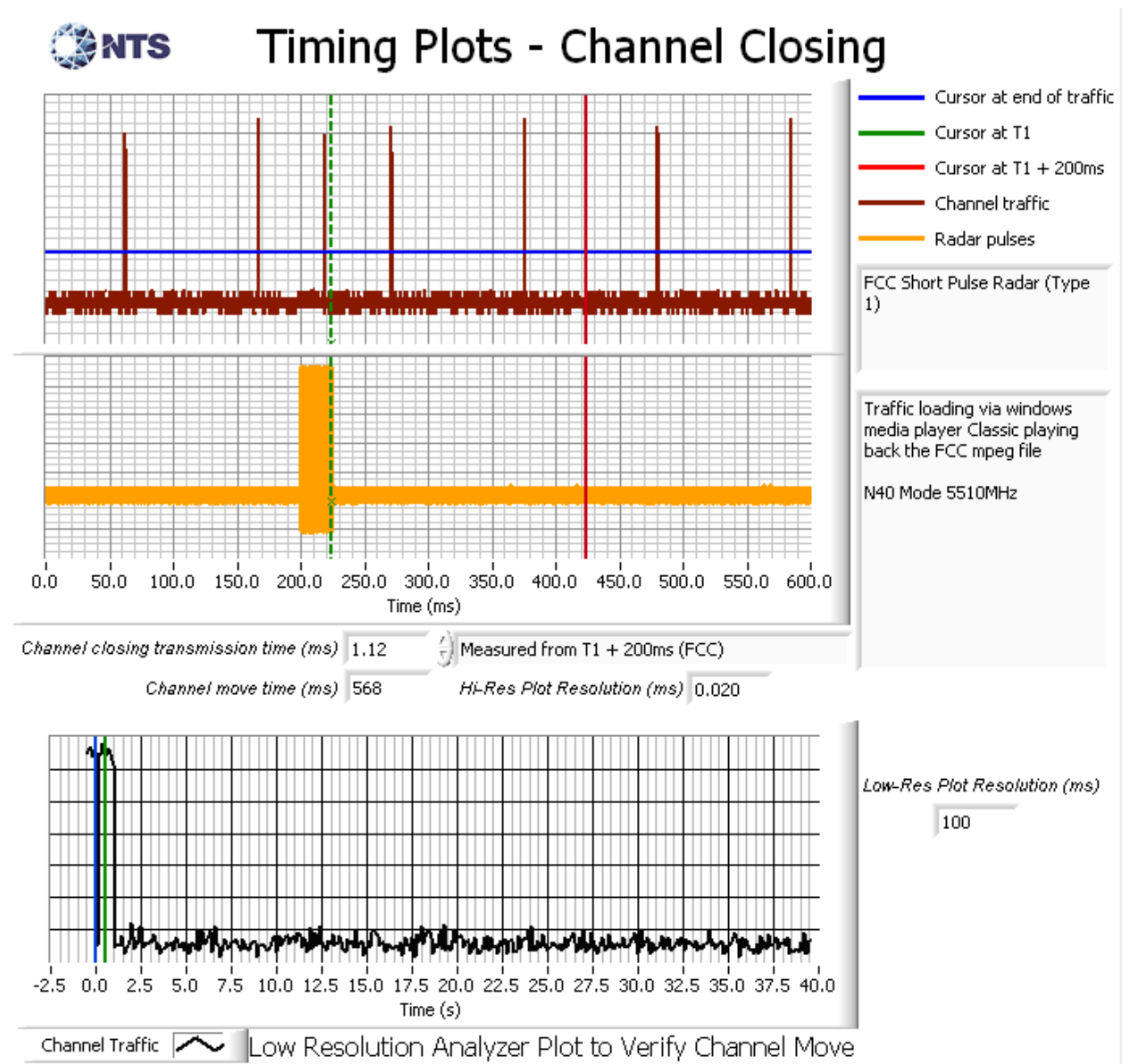
Figure 5 Close-Up of Transmissions Occurring More Than 200ms After The End of Radar
