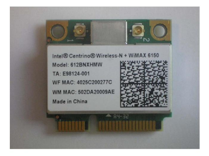
Photo showing label placement on half-mini card.
