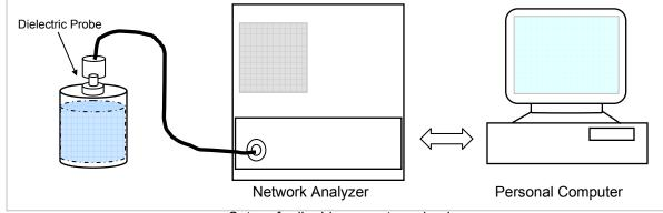
Set-up for liquid parameters check
