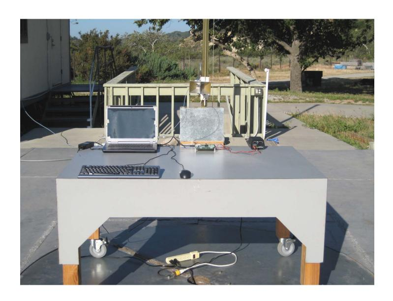
Radiated Emissions Measurement (Front View) WiMax Setup
