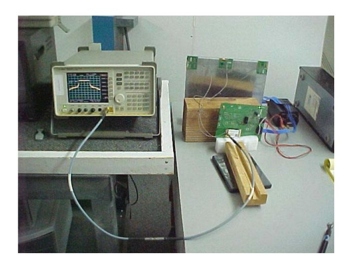
Conducted Emissions at Antenna Terminal Setup
