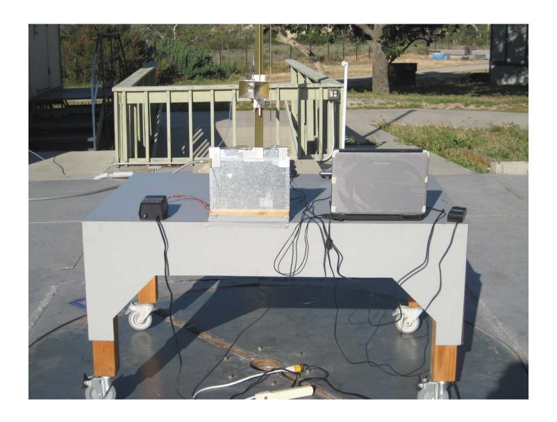
Radiated Emissions Measurement (Rear View) WiMax Setup
