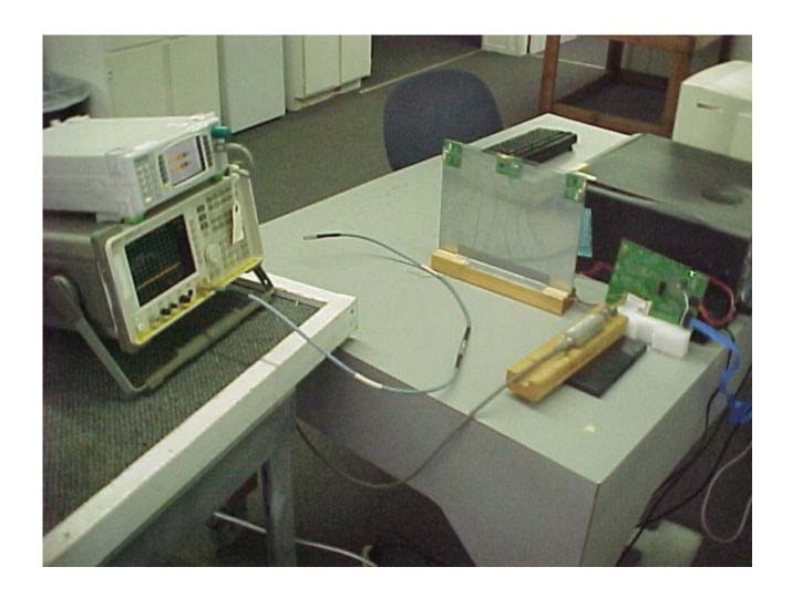
Maximum Peak Output Power Measurement Setup
