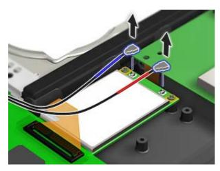
7. Remove the screws that secure the card.
