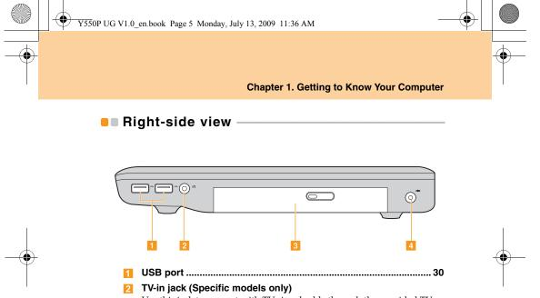
Use this jack to connect with TV signal cable through the provided TV adapter (Analog/digital input supported).
