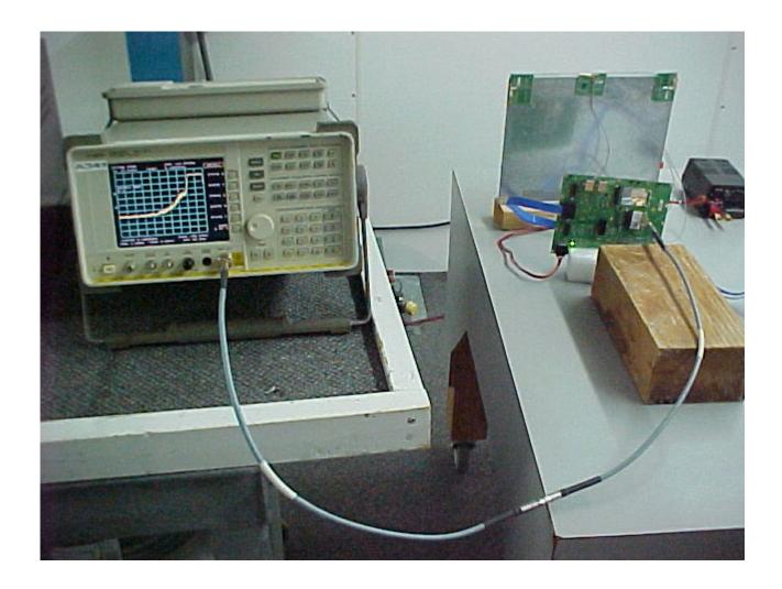
Conducted Emissions at Antenna Terminal Setup
