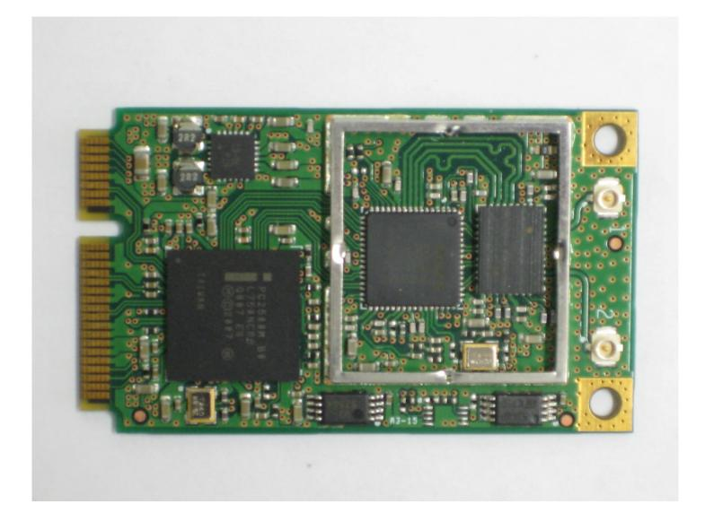
Top View "Shielding fully removed"
