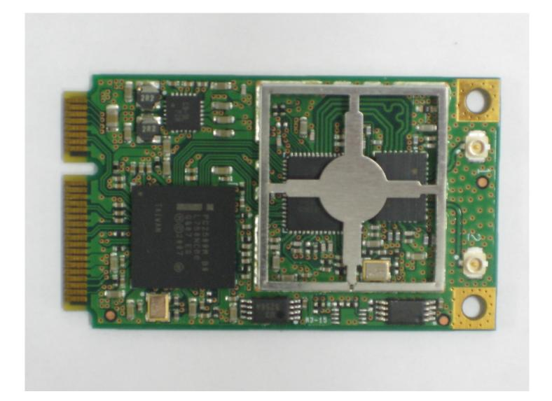
Top View "Shielding partially removed"
