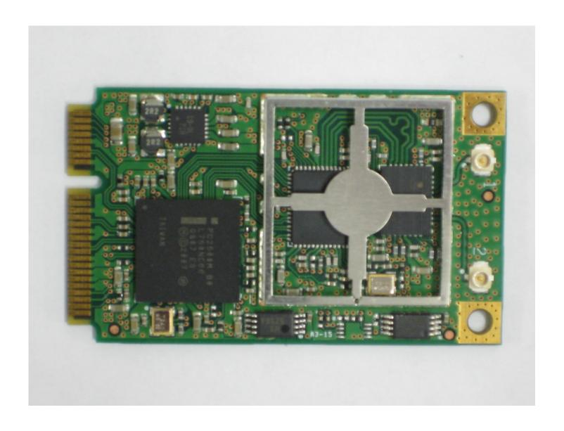
Top View "Shielding removed"
