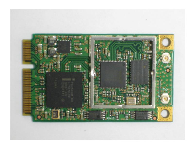
Top View "Shielding completely removed"
