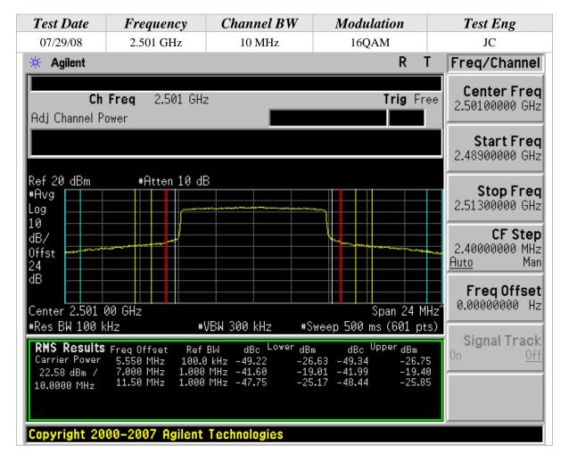
The RF output of the transmitter was connected to the input of the PSA spectrum analyzer through sufficient attenuation.
