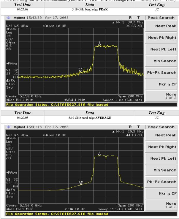
Note: Tested at 16.5dBm with lower internal attenuation – PASS
