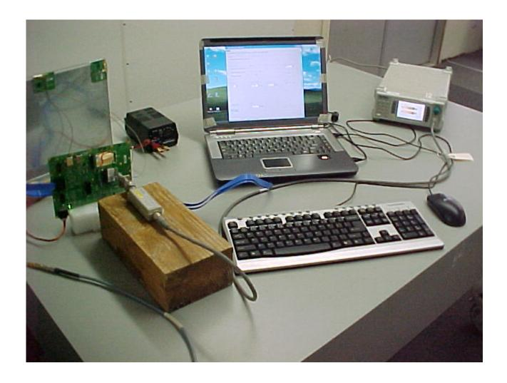
Maximum Peak Output Power Measurement Setup
