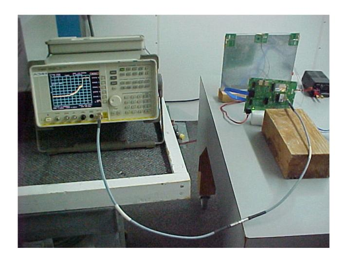
Conducted Emissions at Antenna Terminal Setup
