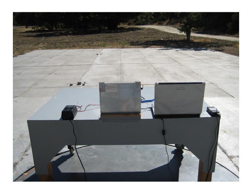
Radiated Emissions Measurement (Rear View) WiFi Setup
