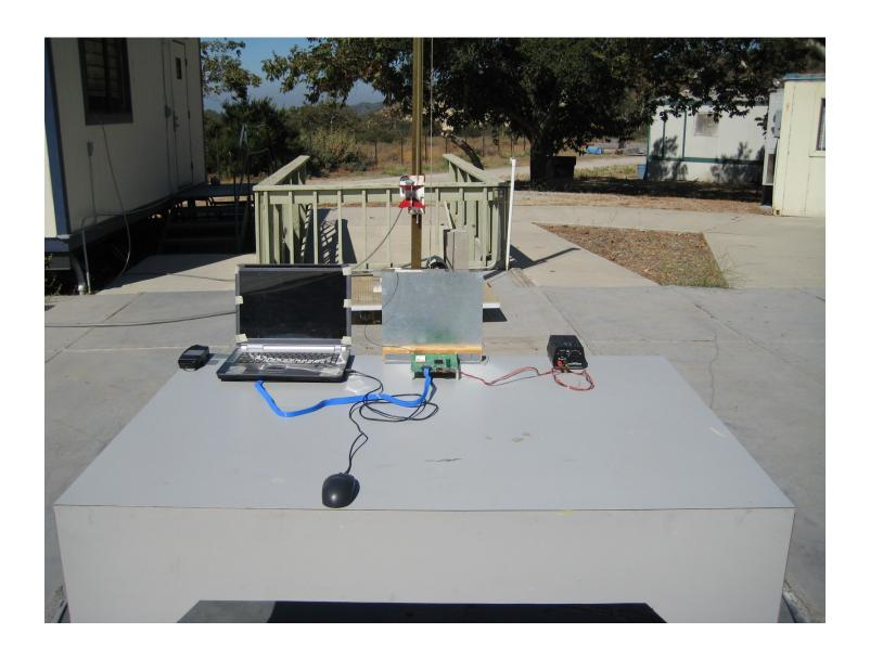
Radiated Emissions Measurement (Front View) WiFi Setup
