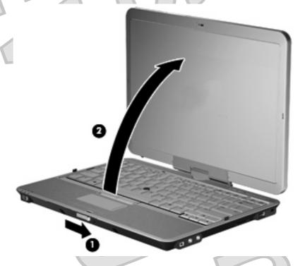
Rotate the computer display counterclockwise until it snaps into place facing the keyboard.
