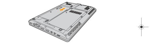
**(5)** Put the battery back in place, turn the computer over again, and reconnect the cables.
