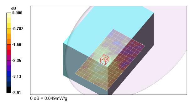
Maximum value of SAR (measured) = 0.049 mW/g
