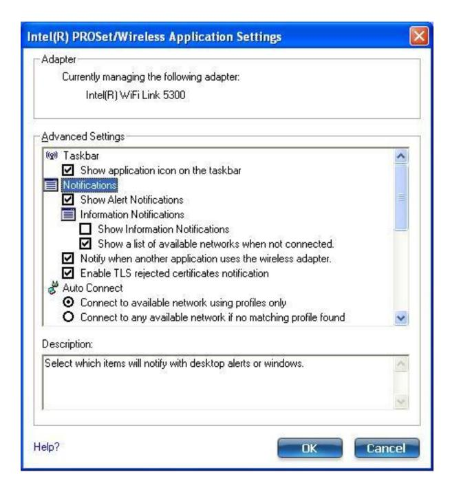
The Application Settings control the behavior of the Intel(R) PROSet/Wireless WiFi Connection Utility.
