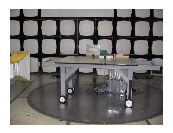
AC Power Line Conducted Emissions Test Configuration Photographs
