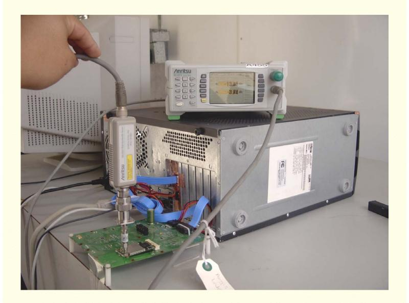
Maximum Peak Output Power Measurement Setup
