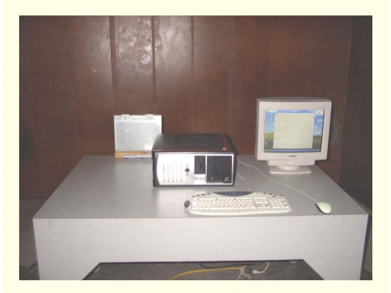
Radiated Emissions Measurement (Front View) Setup
