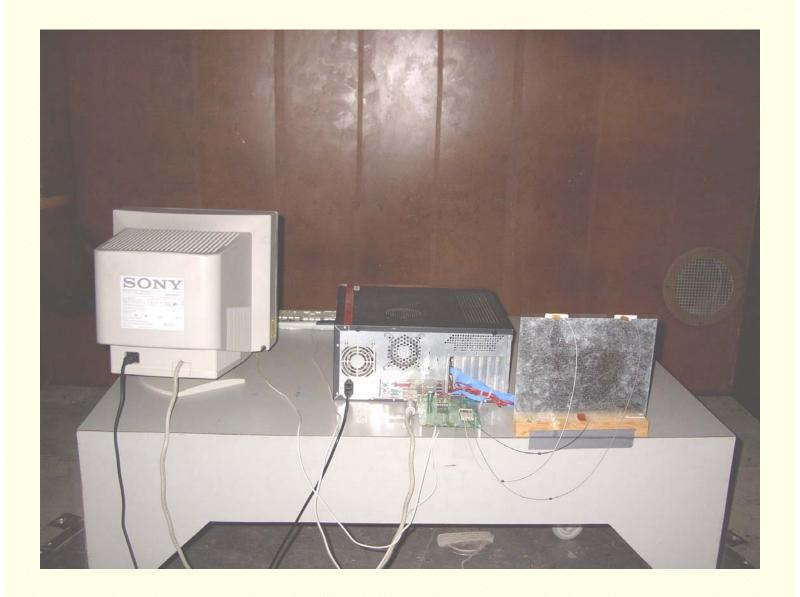
Radiated Emissions Measurement (Rear View) Setup
