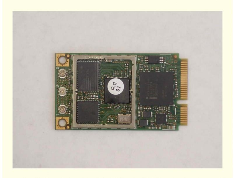
Top View "Shielding removed"
