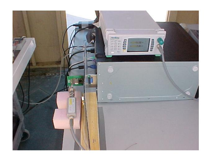
Maximum Peak Output Power Measurement Setup
