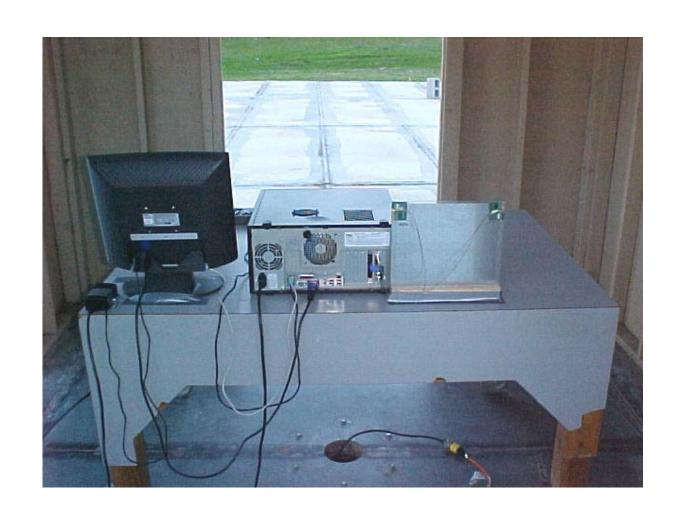
Radiated Emissions Measurement (Rear View) Setup
