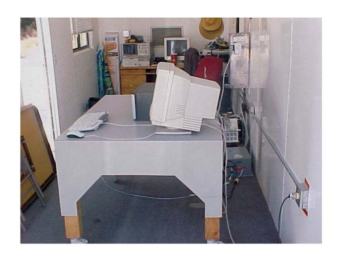
AC Conducted Emissions Measurement (Rear View) Setup
