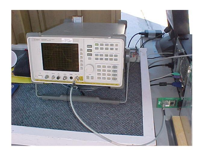
Conducted Emissions at Antenna Terminal Setup
