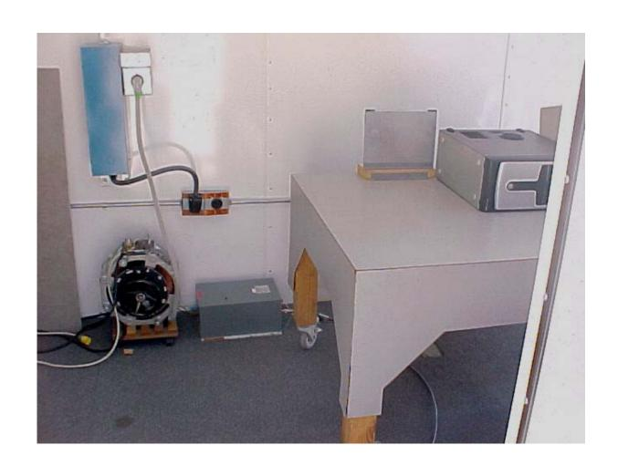
AC Conducted Emissions Measurement (Front View) Setup
