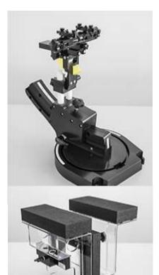
The DASY device holder is designed to cope with the different positions given in the standard. It has two scales for device rotation (with respect to the body axis) and device inclination (with respect to the line between the ear reference points). The rotation center for both scales is the ear reference point (ERP). Thus the device needs no repositioning when changing the angles.
