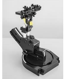
The DASY device holder is designed to cope with the different positions given in the standard. It has two scales for device rotation (with respect to the body axis) and device inclination (with respect to the line between the ear reference points). The rotation center for both scales is the ear reference point (ERP). Thus the
