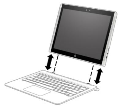
To remove the tablet from the keyboard base:
