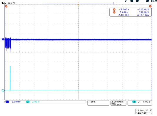
The upper trace in the above plot has 10 seconds of EUT final transmission data and the lower trace shows the simulated radar signal.
