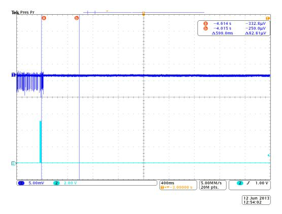
This plot provides a zoom-in to show the 600 ms time interval after the radar burst. This shows that there were not any transmissions after 200 ms following the radar burst.
