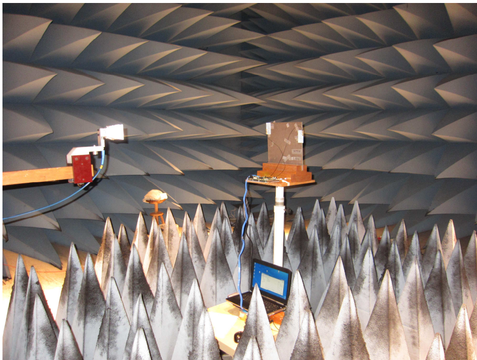
Fig. 4. Test set-up for radiated measurements above 30MHz to 18GHz
