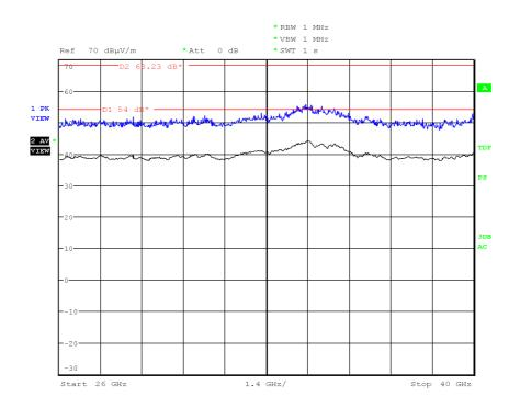
No spurious signals were found in all modulations and channels tested.
