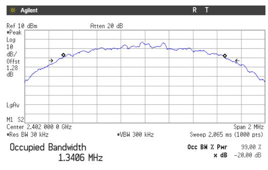
Transmit Freq Error -6.008 kHz x dB Bandwidth 1.448 MHz
