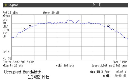
Transmit Freq Error -6.958 kHz x dB Bandwidth 1.439 MHz
