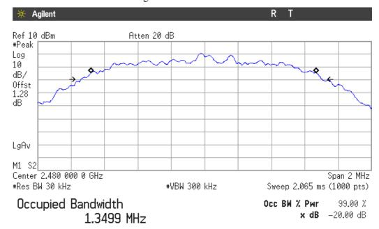
Transmit Freq Error -6.615 kHz x dB Bandwidth 1.442 MHz
