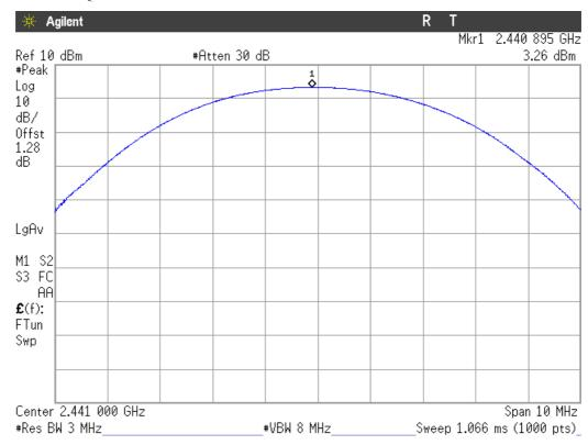
Modulation: Π/4-DQPSK Highest Channel: 2480 MHz.
