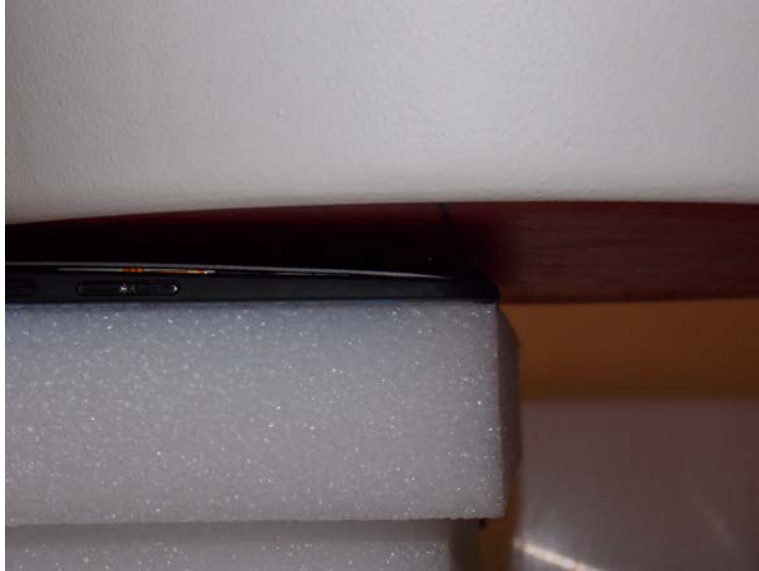
Test Position Back Both Antennas 0 mm Gap
