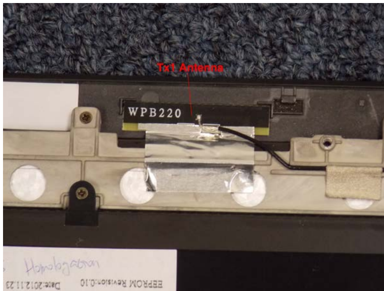
Close up of Tx1 Antenna
