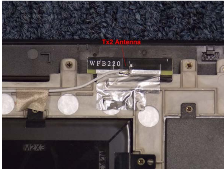
Close up of Tx2 Antenna
