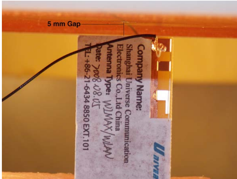
Test Position Side C 5 mm Gap
