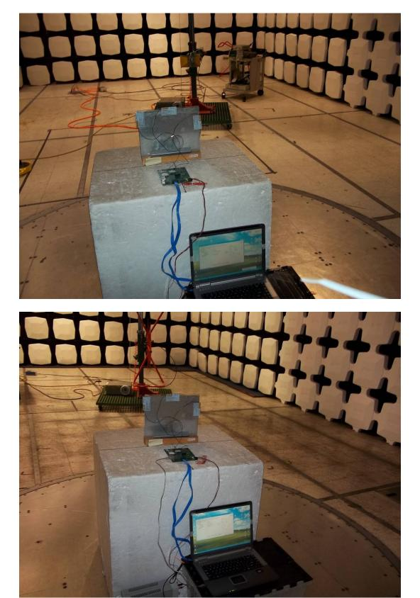
Radiated Emissions Test Configuration Photographs
